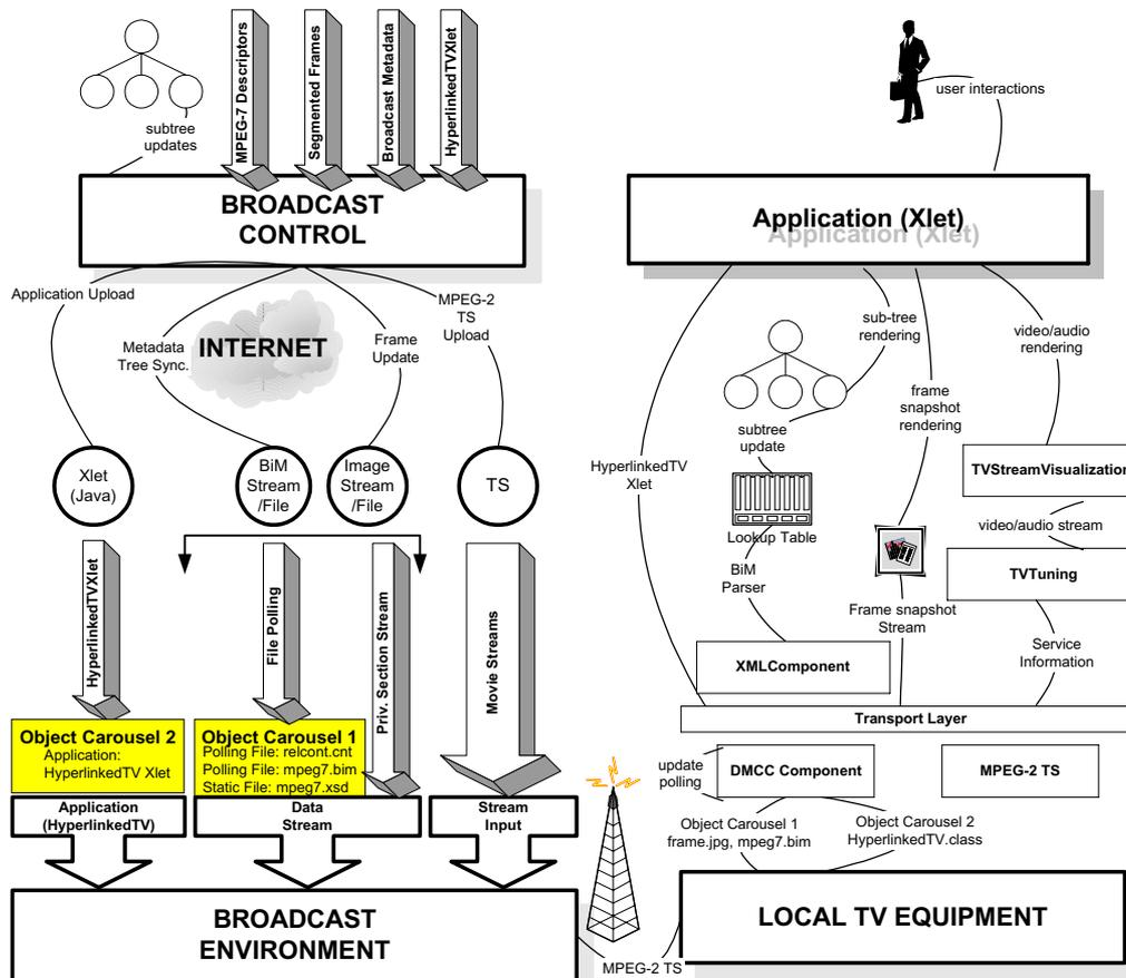
Figure 4. Broadcast-, and client architecture flow diagram.
