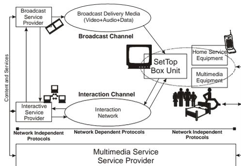
**Figure 1.** Generic service architecture for service provision on the digiTV platform.
